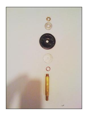
**7.** To remove flow control stem from top, first use a flathead screwdriver to turn the flow control stem as many turns as possible in clockwise direction. Next, unscrew the flow-control stem from the underside of the top.
