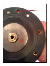
**PROBLEM:** Water leaks out of top of adaptor where flow control stem protrudes from top housing.
