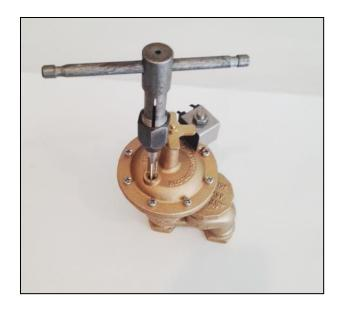
**PROBLEM:** Water leaks out of adaptor between top and lower section and tightening top screws does not stop leakage.
