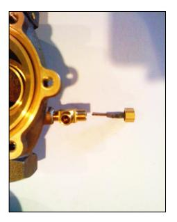
**7.** To remove flow-control stem from bonnet, first rotate cross-handle clockwise as many turns as possible, then remove nut and cross-handle from top of stem. Next, unscrew flow-control stem from underside of bonnet.
