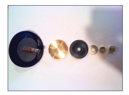
**5.** Photo below shows completely disassembled diaphragm assembly. From top to bottom: Diaphragm shaft, fiber washer, upper diaphragm plate, diaphragm, lower diaphragm plate, fiber washer, spacer nut, fiber washer, disc holder, rubber seat disc, retaining washer, retaining nut, and cap.
