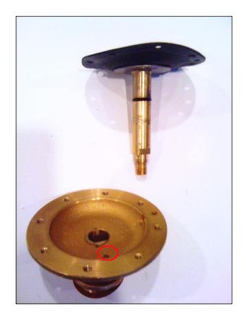
**PROBLEM:** Valve will not close and a steady stream of water exhausts to atmosphere from a port in lower diaphragm housing under the solenoid.
