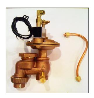
**2.** Using a ½" wrench, remove coupling and L-fitting from solenoid post. Next, slide U-frame and coil off of solenoid post.
