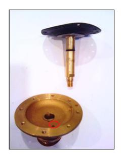
**PROBLEM:** Water leaks out of area where flow-control stem protrudes from top of valve.
