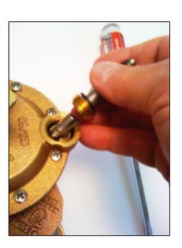
View of solenoid cavity. Note o-ring seal at bottom of cavity. The port in the center of the cavity is the exhaust port leading to exterior of valve. When the solenoid is energized, the water in the upper diaphragm assembly exhausts to atmosphere. About a quarter cup of water will exhaust, then stop. The other port connects the diaphragm assembly to the solenoid cavity.
