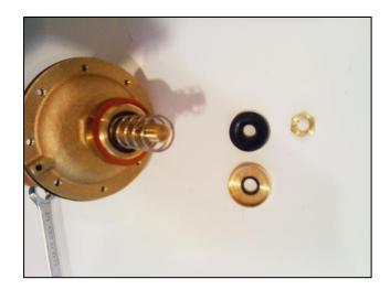
**PROBLEM:** Valve will not close and water continuously exhausts from vent hole in lower section of actuator.
