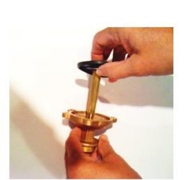
6. To disassemble diaphragm assembly, use a 7/16" wrench to hold shaft, and 9/16" wrench to remove nut at top of diaphragm shaft.
