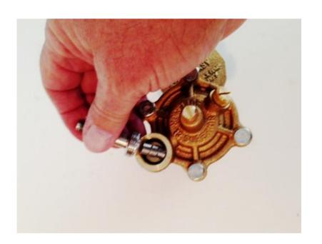
Solenoid cavity: The center port is the exhaust port. The other port connects the solenoid cavity to the diaphragm chamber.
