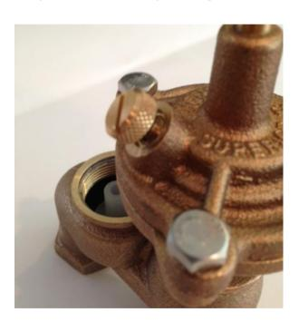
4. Apply a wrench to hex portion (neck) of adaptor and unscrew it from the valve body.
