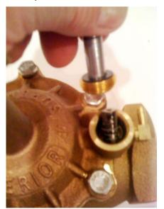
**6.** The photo shows the solenoid cavity of the model 3300. The port directly to the right of the exhaust port (center port) serves no function. The port directly above the exhaust port in this photo leads to the lower diaphragm chamber. The exhaust port leads to the barbed L-fitting where water in lower diaphragm chamber exhausts to atmosphere when solenoid is energized.
