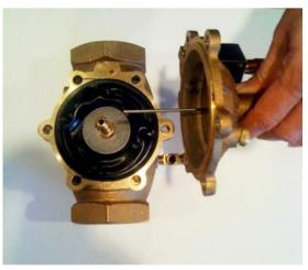
**4.** Remove chamber-plate assembly from valve body.
