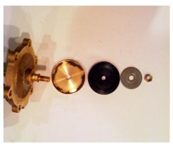
**6.** To access shaft o-ring, first follow step 5 instructions then remove diaphragm shaft from chamber-plate.
