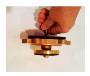
**5.** To remove rubber seat disc from chamber-plate assembly, use a 9/16" wrench to remove nut at bottom of diaphragm shaft and remove retaining washer, rubber seat disc, and disc holder.
