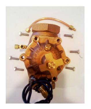
**3.** Lift top straight up and off of body and chamber- plate assembly taking care that metering rod clears the top of the diaphragm shaft.
