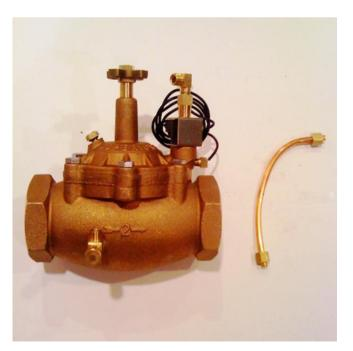
**2.** Remove bolts that fasten top to body and chamber-plate assembly.
