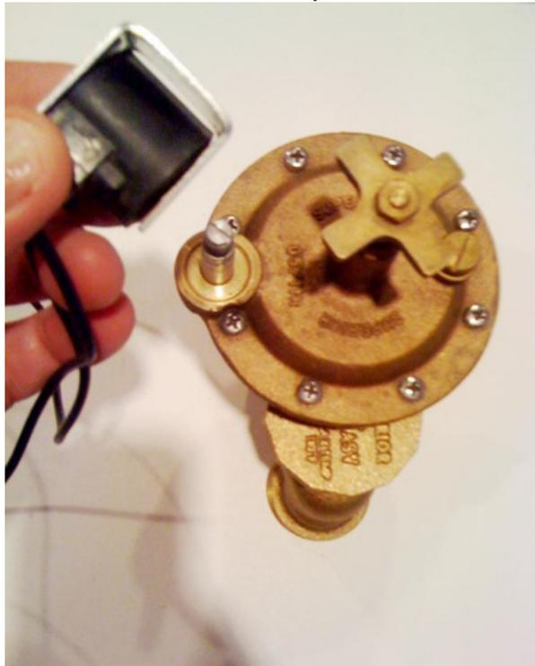
2. Using channel locks, remove anti-siphon cap from valve body.
