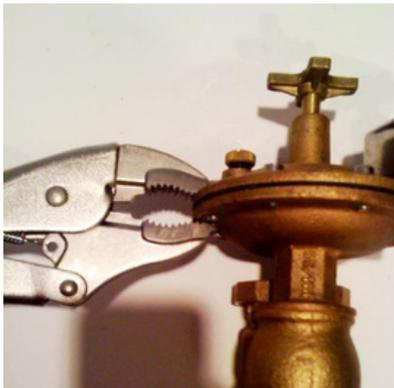
**PROBLEM:** Water leaks out between adaptor and anti-siphon body.
