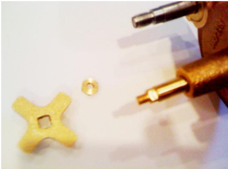
8. Unscrew flow control stem from under side of top.
