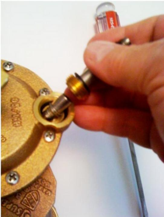
**Solenoid cavity:** The center port is the exhaust port. The other port connects the solenoid cavity to the diaphragm chamber.
