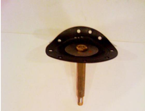
6. To disassemble diaphragm assembly, use a 7/16" wrench to hold shaft, and 9/16" wrench to remove nut at top of diaphragm shaft.
