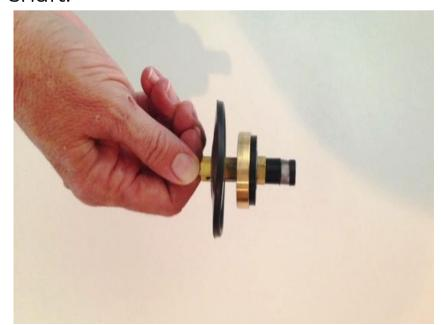
**8.** For 950DW, 950DWIB, and 950PRS models, unscrew filter from bottom of shaft.
