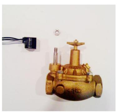
2. Unscrew bolts that fasten valve bonnet to valve body.
