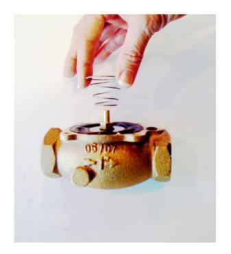
**5.** Remove diaphragm assembly from valve body.
