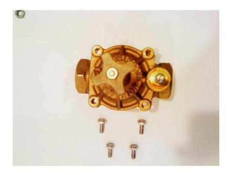
**3.** Lift bonnet straight up off of valve body taking care that the metering in bonnet exits top of diaphragm shaft.
