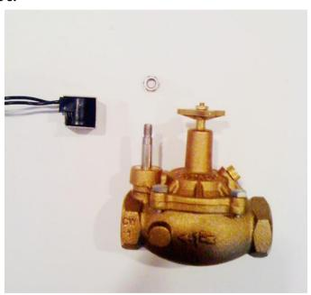
2. Using a flathead screwdriver, unscrew and remove solenoid post from top of valve.
