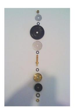
8. To remove flow control stem from bonnet, remove nut and cross-handle from top of stem, then unscrew flow control from underside of bonnet.
