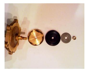
**6.** To gain access to shaft o-ring, remove diaphragm shaft from chamber-plate after the seat disc and disc holder have been removed from bottom of shaft.
