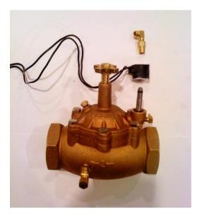
**4.** Using a flathead screwdriver, unscrew solenoid post from bonnet.
