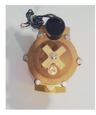
2. Take care as you remove the solenoid as the solenoid plunger will drop out of plunger tube.
